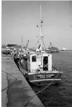
The Blucher, a GRP boat made from a mould of the William Edward.
