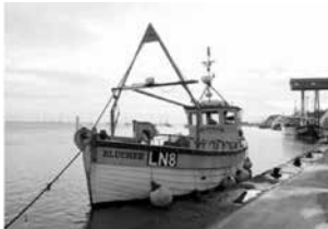
The Blucher, a GRP boat made from a mould of the William Edward.
